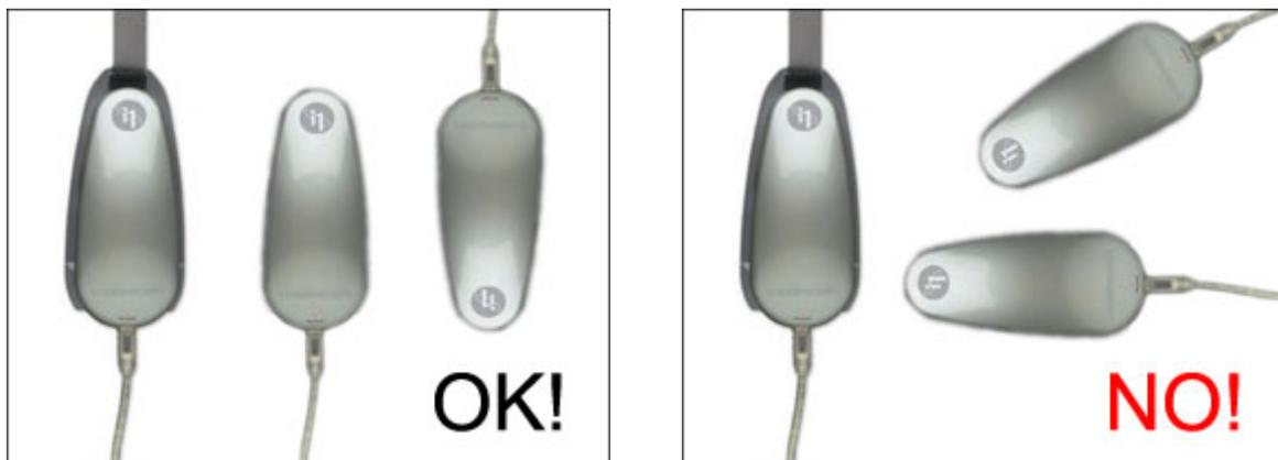
**Note:** "Older" CRT displays do not emit polarized light and are thus not susceptible to errors due to instrument orientation. As for the Eye-One Display and the Spyder2 colorimeters, their simpler optical layout makes them immune to this effect.
